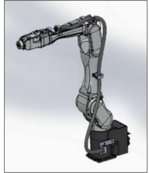
51.29.001.01 Complete robotic dresspack, Axis 1-6, without retraction system, high-flex conduit with ID 23.1mm
